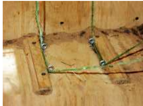
Figure A-3. A view of the four eye-bolts at the bottom of the baler that are important to hold the string in the proper alignment as the pine straw is loaded and compressed.
