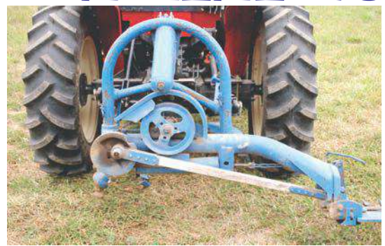
Pitman bar made of wood, so that it CAN break.
