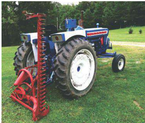
Sickle-bar in raised position for transporting.
