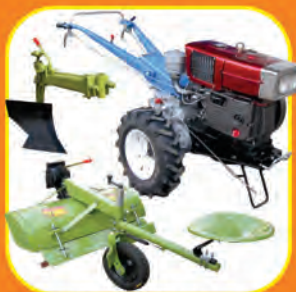
9kW 2-wheel tractor with plough and rotavator
