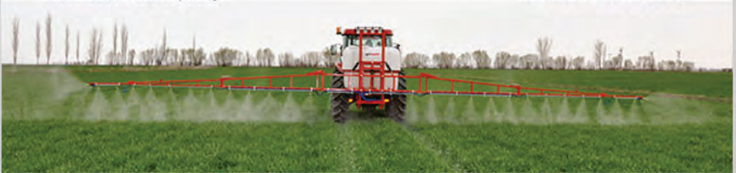
Mounted Boom Sprayer 600-1000 Litre capacity
