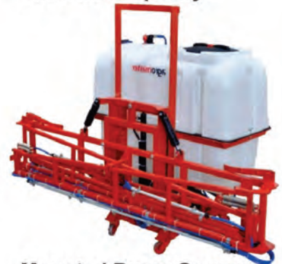
Mounted Boom Sprayer 600-1000 Litre capacity
