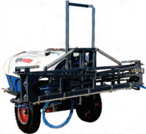
Trailed Boom Sprayer 1000-2000 Litre capacity
